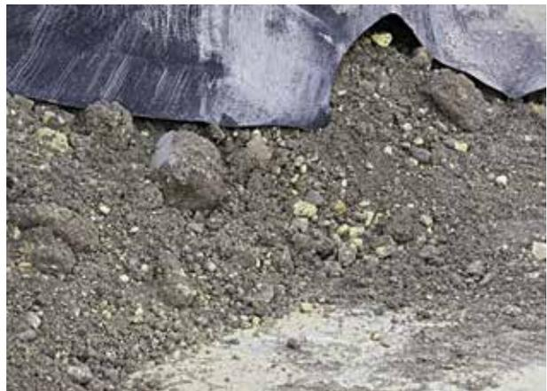
**Figure 4.** Test 1 raw material (approximately 80% sulfur content).
