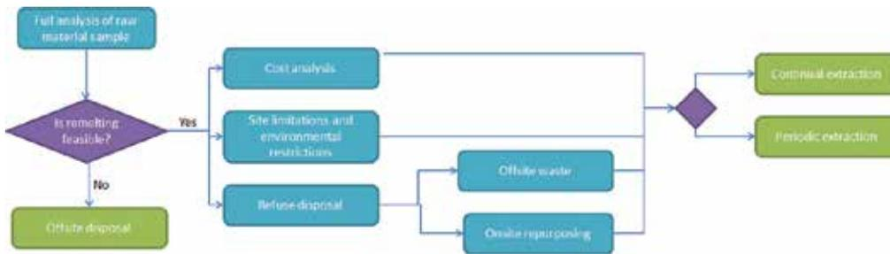
**Figure 6.** Decision tree for contaminated sulfur disposal.
