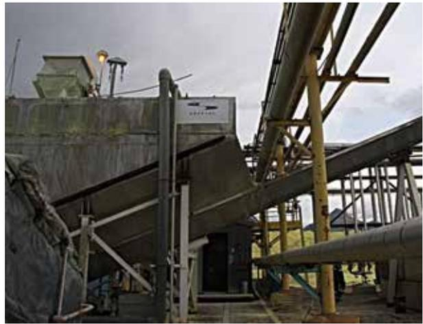
**Figure 3.** Enersul's HCSR remelter.
