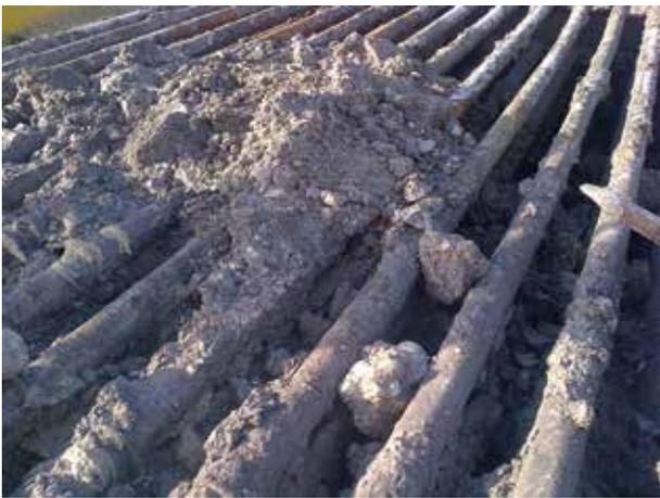
**Figure 2.** Remelting pit heating coils covered with contaminant.
